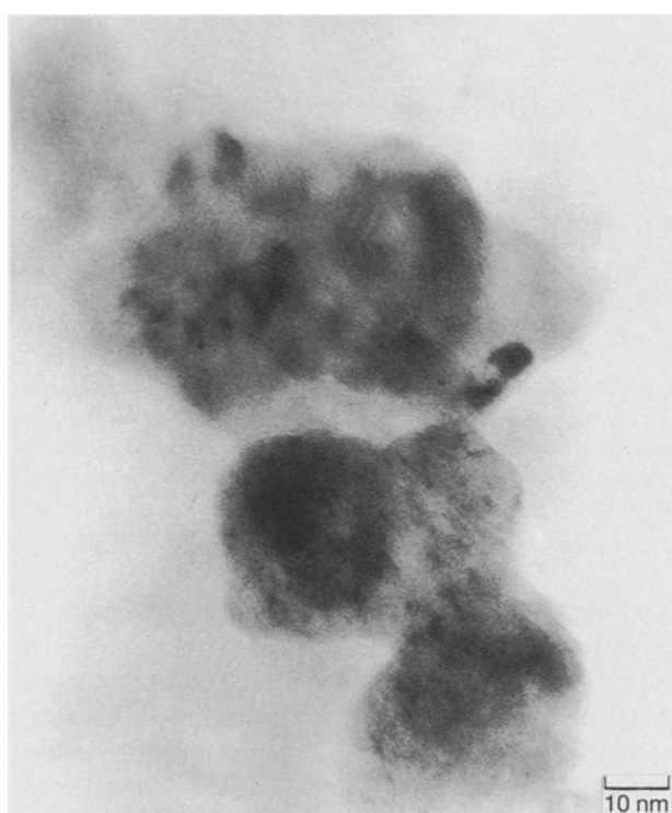
Figure 29 Transmission electron micrograph showing the ultrafine ( \approx 20 nm) particles of the oxysulphide precursors used to synthesize \beta\text{-La}_2\text{S}_3 .
