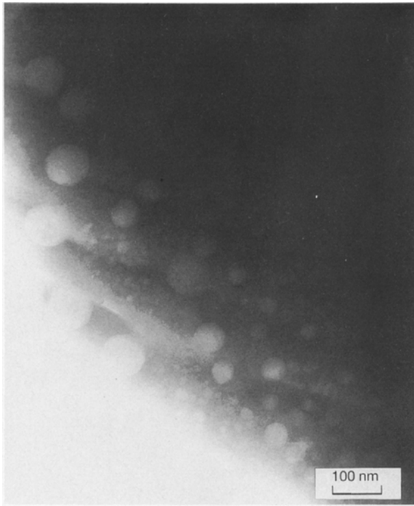
Figure 11 Transmission electron bright-field image showing primary phase-separation in glasses containing 92.5 mol % \text{GeS}_2 . Note the presence of glass droplets in the size range of 6–88 nm distributed in the glass matrix.
